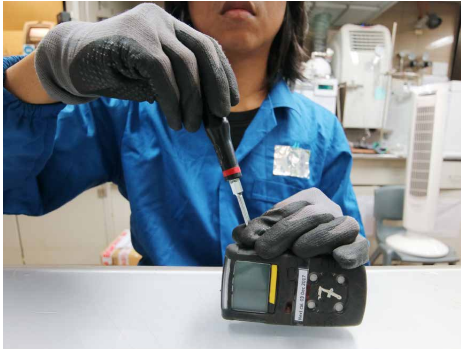
Gas detector maintenance
